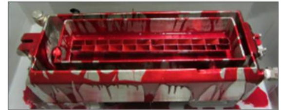
Artificially 'contaminated' production part ready to perform 1 st cleaning trials
