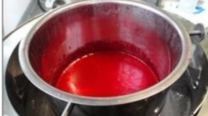
'Placebo' contamination simulation, using "coloured" gelatine for R&D cleaning trials
