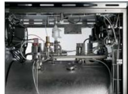
Modulating valve on steam inlet
